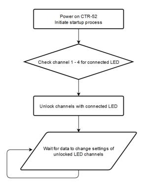
Figure 1 - Startup process CTR-52
